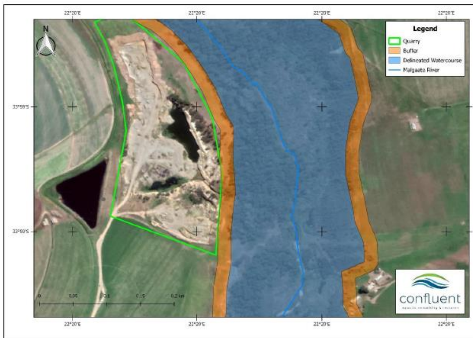
Figure 9: Map illustrating the prescribed buffer zone of 20 m in relation the watercourse and its delineated riparian zone and the quarry.
