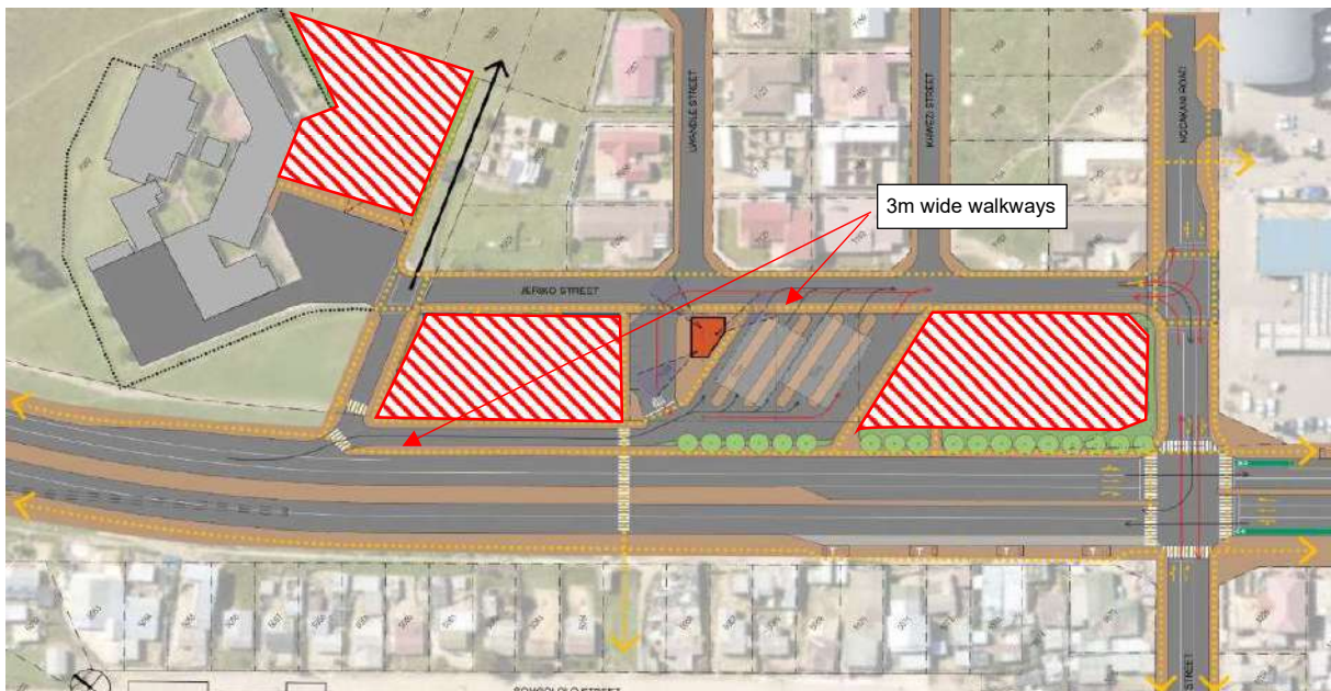
Figure 6.9: Pedestrian access to the Transfer Location
