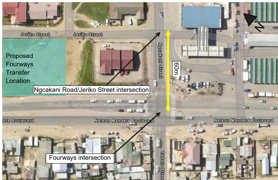
Figure 6.6: Spacing of Ngcakani Road / Jeriko Street and Fourways signalised intersections
