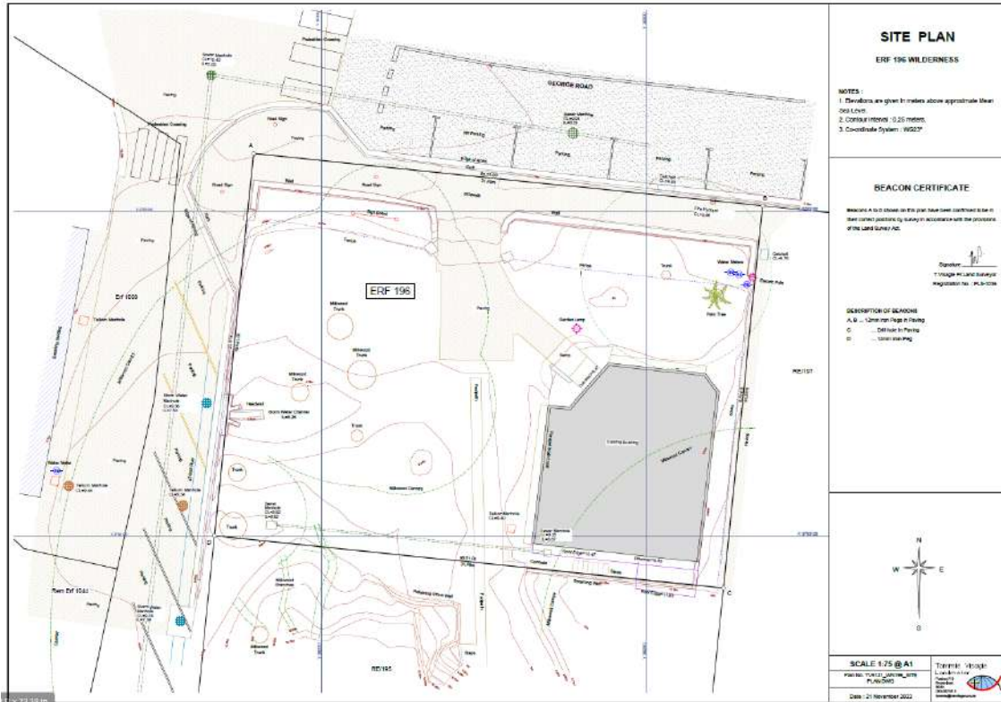
Proposed site plan showing the existing building and associated infrastructure and surveyed protected trees and canopy cover
